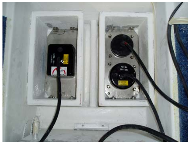
Furuno 2kW hi performance BLT series transducers mounted in hull providing depth range to 2,000m.
