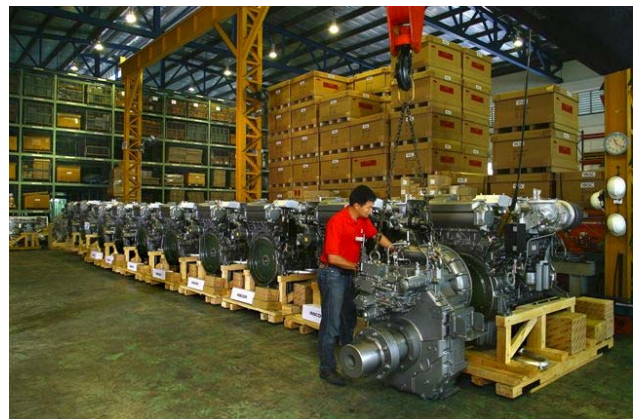
6AY Units fitted with 6:1 reduction gears being prepared for delivery ex Singapore warehouse for local tug boat applications
