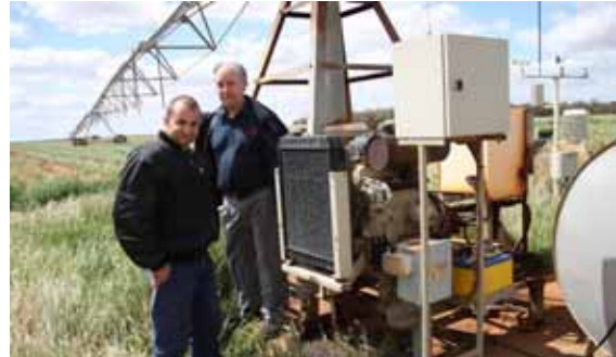
John Lamattina (L) with David Trebilcock of Power Equipment alongside the Yanmar 4TNE88 diesel engine that has logged 15,000 hours in 10 years.
